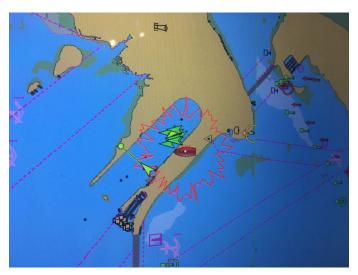
This is what the AIS MOB signal looks like on a chart plotter when the AIS FLARE ECO is activated. The jagged red "circle" flashes and rotates to draw attention to the MOB alert.
