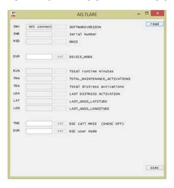
If the app is loaded successfully then you will have this programming page. Hold the android device very near/on top of the MOB and click "read" in the top right corner.
